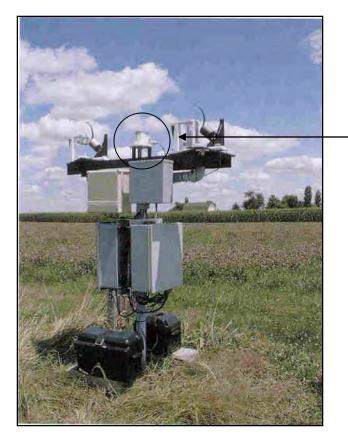
Broadband UV meters measure ultraviolet radiation in the UV-B spectral range of 280-330 nanometers.
